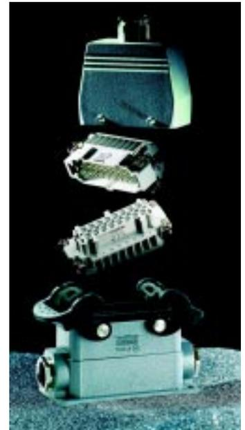
Within the PROCON multipole heavy duty connector system one housing is not assigned to only one series. It can accommodate female or male inserts of different series. Housings for female or male contact carriers are used instead of plugs and sockets. Therefore in a not completely enclosed environment the designer can place the partly live contacts into a female insert.
